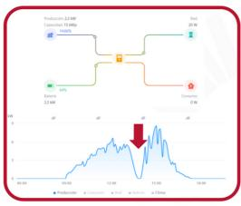
**Inverters and optimizers** can give some information about the status of the plant automatically, but they only measure instant production, which is not enough or specific data for diagnosis.
