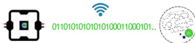
Information is sent to cloud using SSL connection trough port #80, #443 and #23. The data provided by measurement device is stored in the cloud server and it is cross-platform accessible. The communication is from inside network to outside, it doesn’t require to modify potential firewalls or security that network installations could have.
